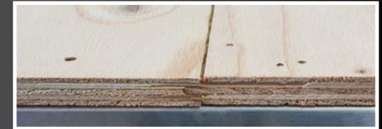
**5/8-INCH TONGUE AND GROOVE PLYWOOD** floor decking.
