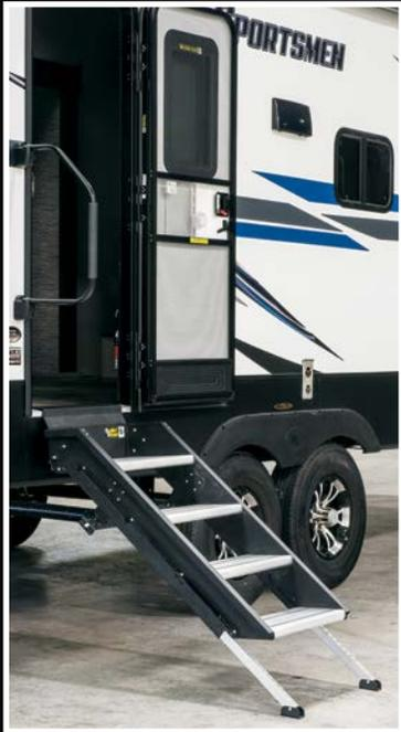
**FLIP-UP ENTRY STEP** provides solid footing and folds away neatly. The friction-hinged entry door with grab bar and screen-shot feature eliminates slamming, for safe and easy passage.
