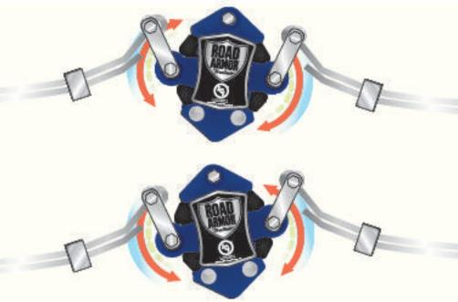
**EXCLUSIVE Road Armor™ Suspension** W/ 360° Vibration Control Equalizes axle load to dampen shock and vibration.
