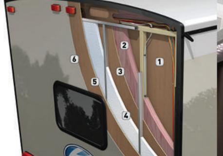
Double-Insulated Laminated Rear Wall (Non Legacy) A Montana EXCLUSIVE and the best insulated rear wall in the industry.
