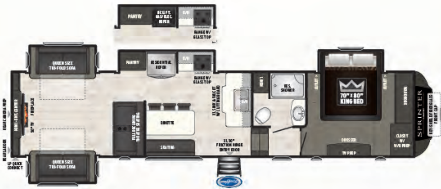
3530/31FWDEN | Rear-den w/ bartop, and both sofas fold out to make ample additional sleeping Weight: 10880 LBS. | Length: 39' 0"
