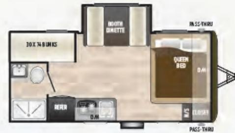
**176LHS** | New single-axle, one slide, double bunkhouse w/ roof mount a/c & 6 cu. ft. fridge
