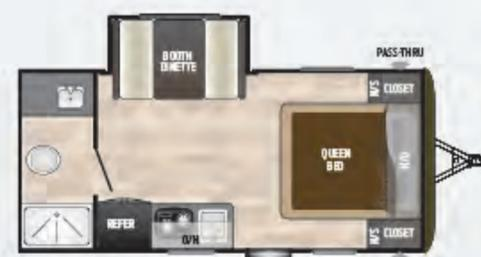
**179LHS** | New single-axle, rear bathroom w/ roof mount a/c and 6 cu. ft. fridge
