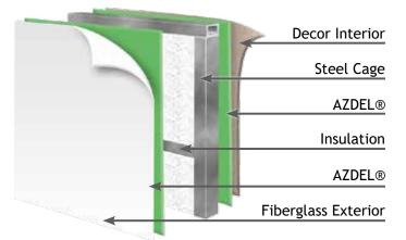
High strength low alloy steel framing throughout motor home — **72% stronger than aluminum!**AZDEL® substrate in sidewalls and roof
