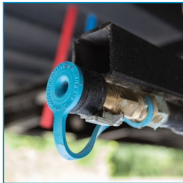
Exterior LP Connection
