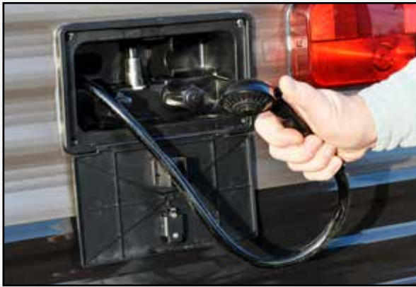
Outside Shower with hot and cold water.
