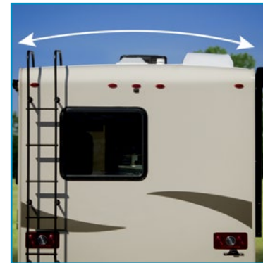
TPO Crowned Roof for Easy Water Runoff
