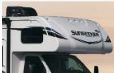
Seamless front cap for enhanced aerodynamics
