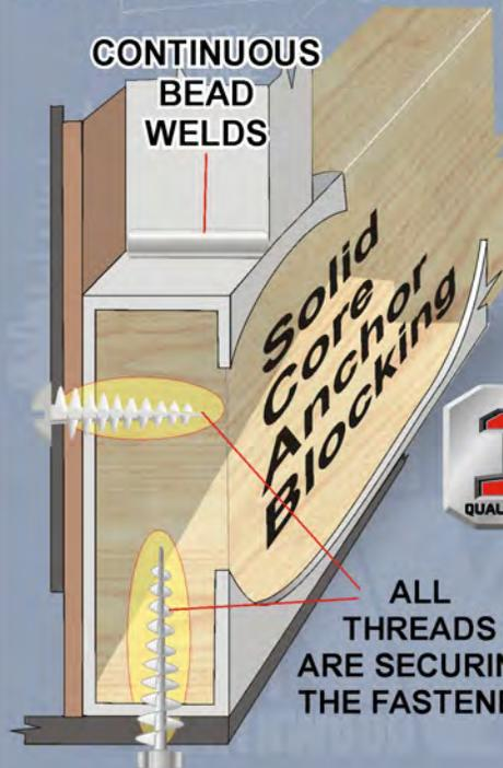
We add solid core anchor blocking in the frame perimeter. The solid blocking provides a substantial anchor medium for securing screws.
