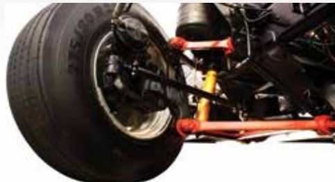
ZF DOUBLE WISHBONE INDEPENDENT FRONT SUSPENSION & PREMIUM SACHS® SHOCKS
