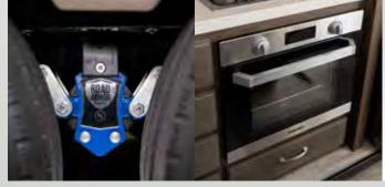
EXCLUSIVE Road Armor™ suspension Equalizes axle load to dampen shock and vibration
