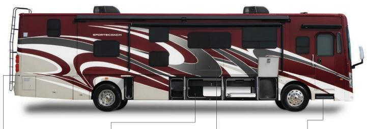
With a 360 horsepower ISB Cummins rear diesel engine and a 6-speed Allison 3,000 MH automatic transmission, Sportscoach gets 800 lbs./ft. of torque and has a 10,000 pound towing capacity.
