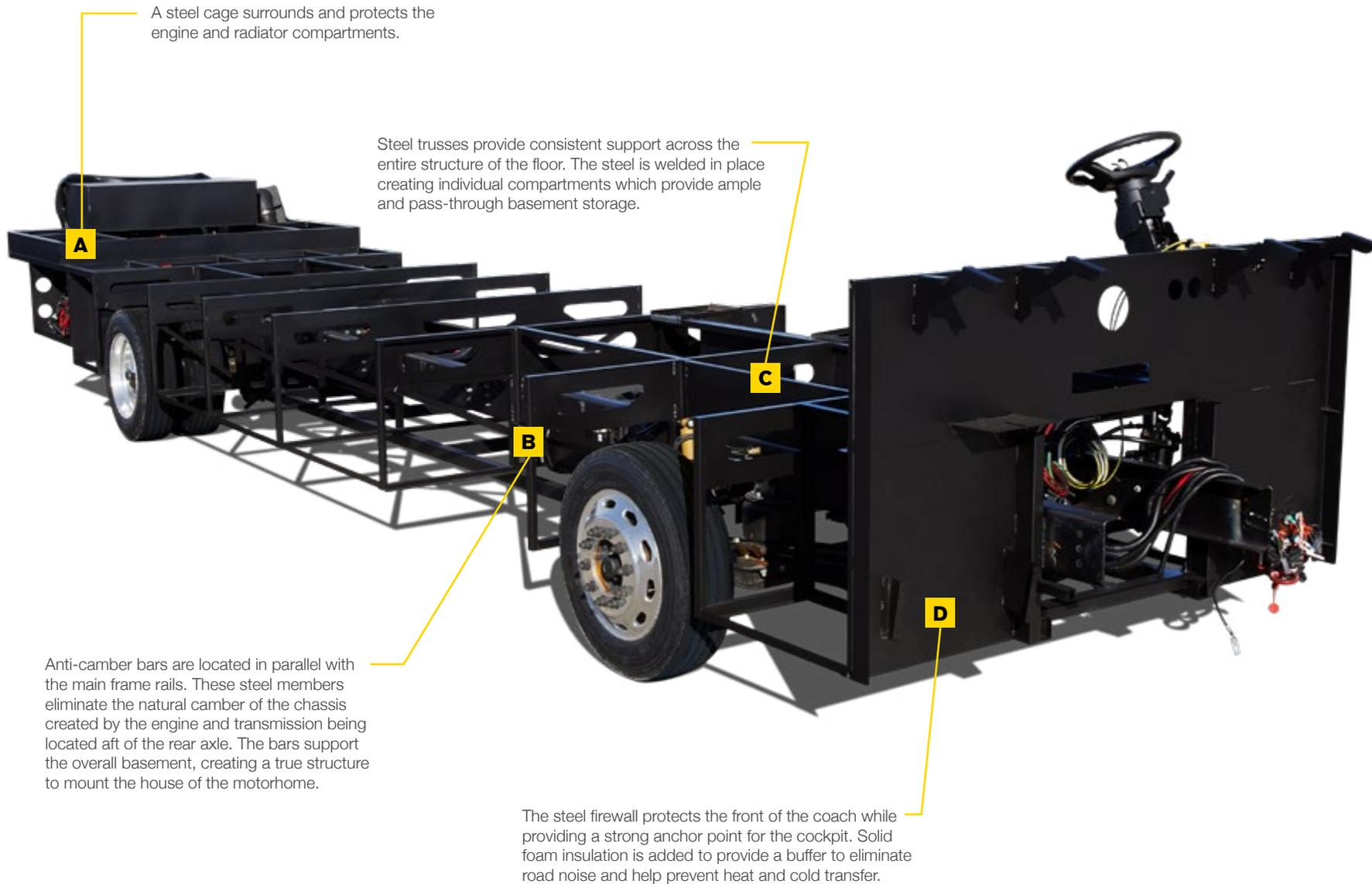
A steel cage surrounds and protects the engine and radiator compartments.
