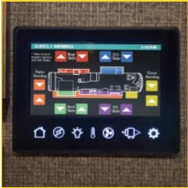
Multiplex Wiring Control System with 7" Touchscreen
