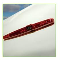
Back-up Monitor with Integrated Rear Camera
