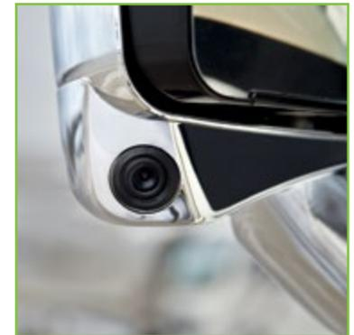
Heated/Remote Exterior Mirrors with Integrated Side View Cameras
