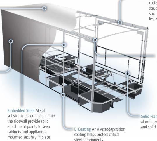
Laser-Cut Tubing Precision laser cutters create precise joints in structural steel that are stronger and require less welding.
