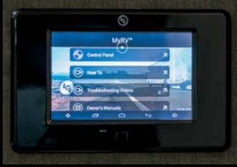
My RV gives you command of your fifth wheel from one location, with the touch of your finger. This allows you to control the awning, landing gear, and slideouts, as well as access to troubleshooting videos and your owners manual (included with optional leveling system).
