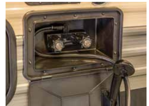
Outside Shower with Hot & Cold Water
