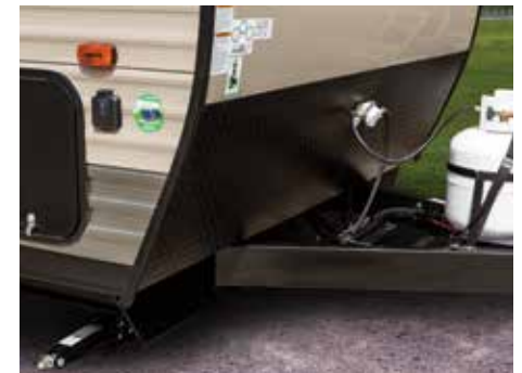
High Impact Front Metal Replaces Corrugated Metal
