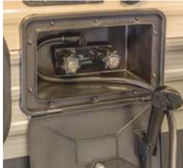
Outside Shower with Hot and Cold Water
