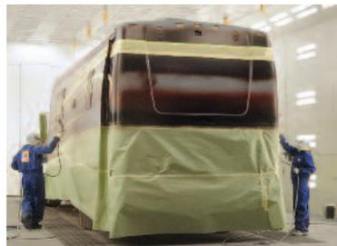
Dynamax has three on-site 25' x 60' downdraft paint booths. This means we have maximum control of quality. By painting parts and slide-outs before they are installed, we eliminate overspray on slide seals and interior components.
