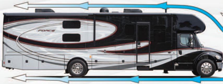
Unlike flat-front, bus-style motorhomes, a Class C utilizes an automotive cab chassis for better airflow, fuel economy, performance, and added safety.
