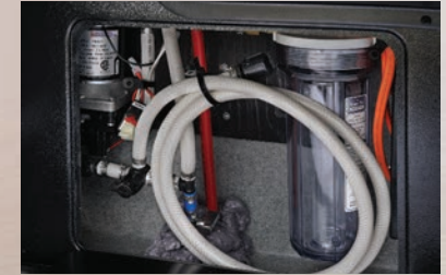
WINTERIZING TUBE Easy access for quick maintenance includes bypass valve.
