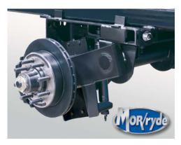
MORryde® I.S. Suspension eliminates the axle and leaf springs, allowing each tire to work independently. With 5 1/2" of travel per assembly, MORryde® I.S. will absorb road shock and protect your home for its lifetime.
