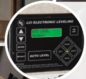
The Ground Control Leveling System, makes leveling your Aerolite easier than ever.
