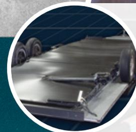
In addition to the leveling jacks, your Aerolite comes with a fully-enclosed underbelly and fully-laminated aluminum frame construction for the best in durability and stability.
