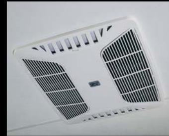
Sidewinder comes standard with 3" x 14" foam-core in-floor straight-line heating system with 35,000 BTU furnace and 15,000 BTU ducted roof air conditioner.
