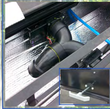
Heated Holding Tanks with Protected Valve System
