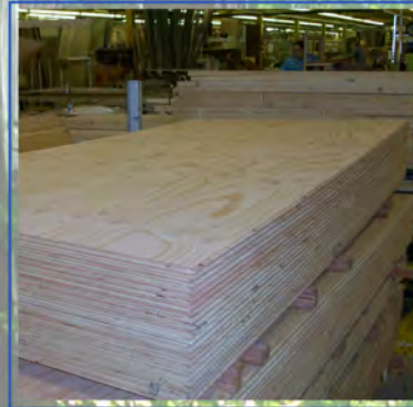
Plywood Roof & Floor Decking
