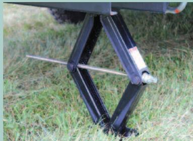
Four standard heavy duty stabilizing jacks
