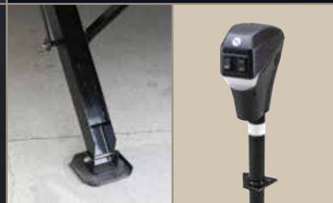
POWER TONGUE AND STAB JACKS POWER TONGUE JACK IS NOT INCLUDED ON 5TH WHEELS
