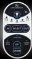
PUSH BUTTON REMOTE OPERATES: AWNING, SLIDES, LED AWNING LIGHTS, POWER STAB JACKS
