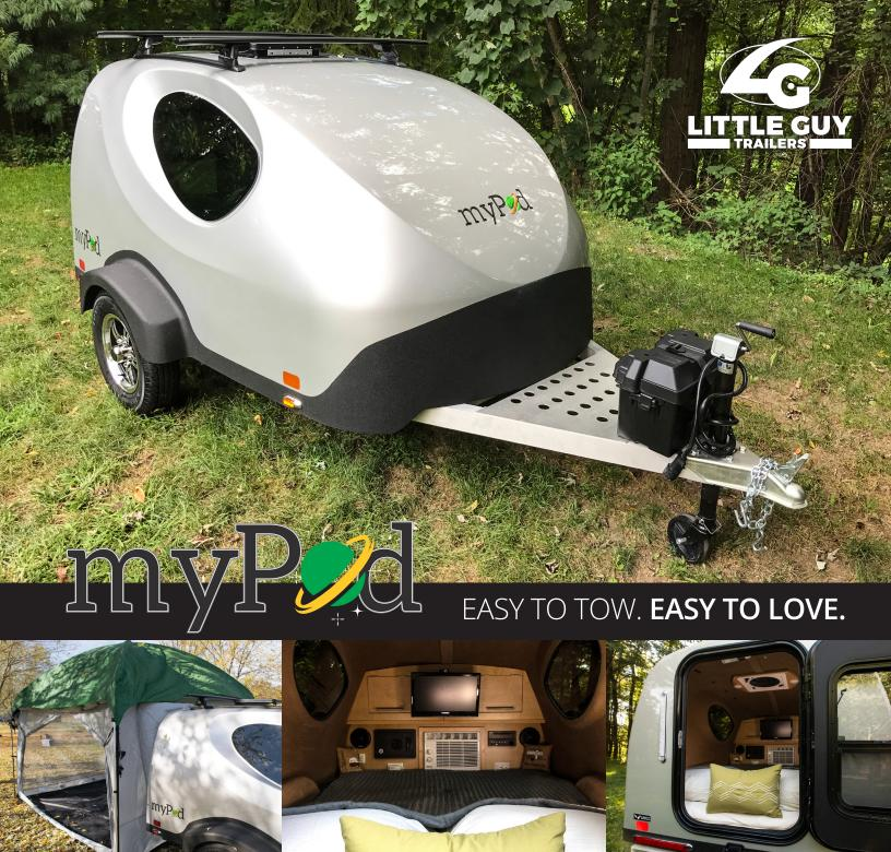
The MyPod is a 100% fiberglass molded body on an aluminum frame. With a dry weight of 630 lbs and tongue weight of just 110 lbs, the MyPod is a perfect for smaller towing vehicles and still packs a ton of great features. Choose from white, silver, black, blue or red. Includes Full/Double Size Bed.
