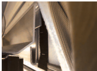
Clipper's exclusive J-Track door latch maximizes stability by eliminating the flimsy nylon turn buttons traditionally used in securing the door to the roof.
