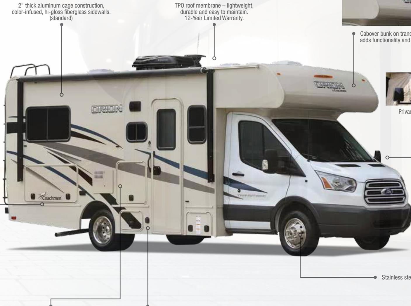
2" thick aluminum cage construction, color-infused, hi-gloss fiberglass sidewalls. (standard)
