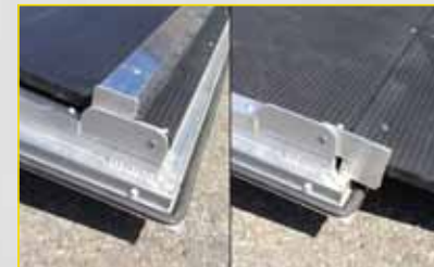
The new FTH (Flat Transition/Hingeless) Flap System makes loading and unloading snowmobiles smooth without sacrificing the ability to load heavier machines/cars when it's not sled season.
