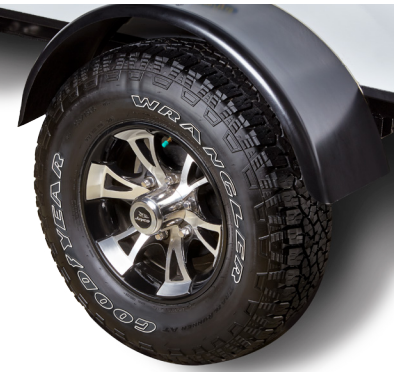
AMERICAN-MADE NITRO-FILLED GOODYEAR® TIRES WITH ALUMINUM RIMS AND SELF-ADJUSTING BRAKES
