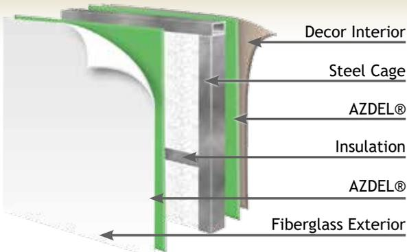
High strength low alloy steel framing throughout motor home – **72% stronger than aluminum!**
