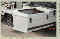
Vikina's Super Sliding Storage box enables full, easy accessibility even when the camper is set up. (Standard on Legend, Optional on V1).
