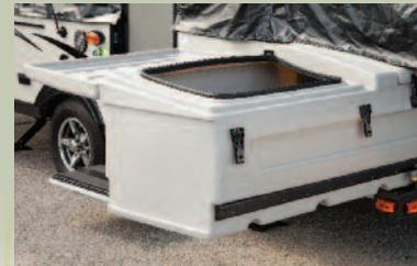
Viking's Super Sliding Storage box enables full, easy accessibility even when the camper is set up. (Standard on Legend, Optional on V1).
