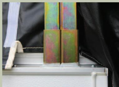
*The Goshen Stamping double-wide lift arm system offers strength, stability and increased wind resistance. (Limited lifetime warranty)*
