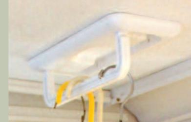
*Retractable clothes bar (Standard on Legend, V-Trec and Hardside models)*
