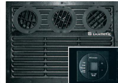
The Dometic Cool Cat 10, 150 BTU heat pump is standard on Viking hardside camping trailers.
