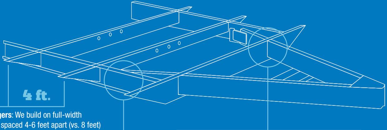
**Full-width outriggers:** We build on full-width outriggers that are spaced 4-6 feet apart (vs. 8 feet) to better support the weight of the wall.
