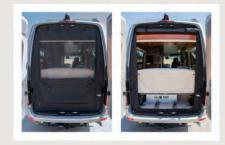
The heavy duty nylon canvas rear roll up screen is available on all our van based models. The double zipper system allows for easy access to the under sofa storage space while the fine mesh screen keeps the insects out and lets the fresh outside air in. The whole screen assembly can be rolled up and tethered out of the way when not in use.
