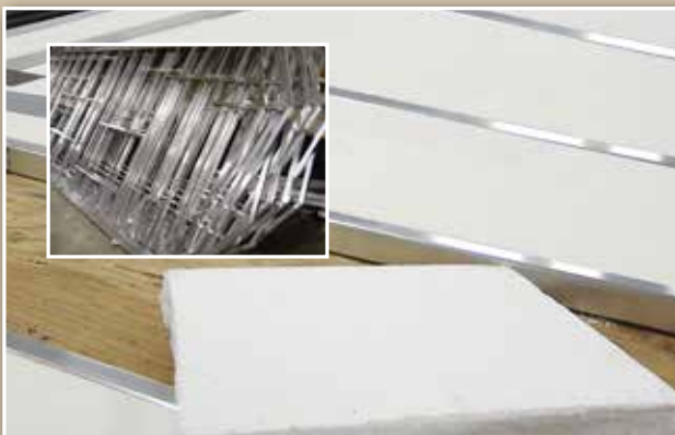
Laminated Sidewall Construction
