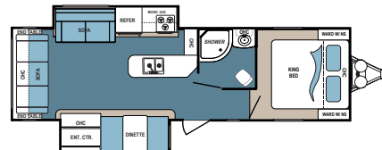
DENALI TRAVEL TRAILER | 2975RL Ext. Length: 33' 9" Ext. Height: 11' 7" Average Shipping Weight: 7,250 Sleeps: 3-4
