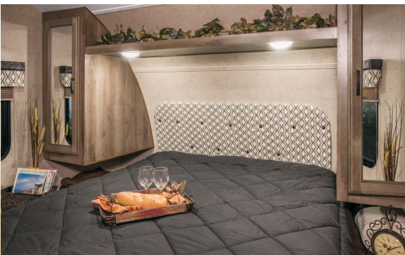
The under-bed storage system is comprised of two baskets on each side, along with under-bed storage, accessed by lifting the 60" x 80" queen bed's plywood base with gas struts.
