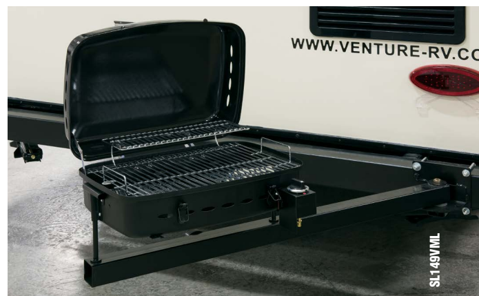
All Sonics feature a square bumper for sewer hose storage, and which can receive an optional bumper-mount grill.
