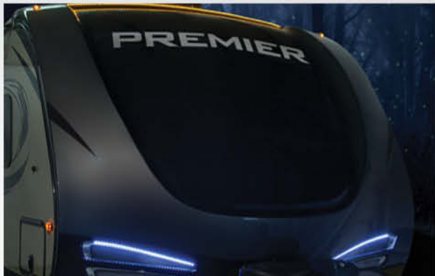
Full Fiberglass Automotive Painted Cap with LED Docking Lights
