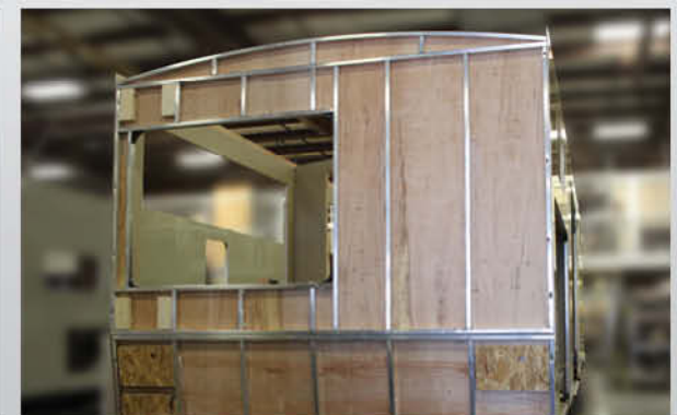
Aluminum Framing Throughout (including slide boxes, pass-thru storage)
