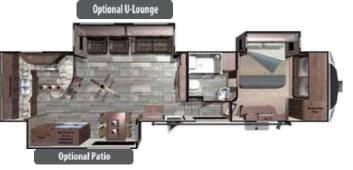
3X388RKS Ext. Length: 39'11" Hitch Weight (lbs): 2,500 Unloaded Wt. (lbs.): 12,280 GVWR: 16,450 Fresh Water (gal): 85 Gray Water (gal): 82 Black Water (gal): 41
