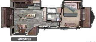
3X349RLS Ext. Length: 37'3" Hitch Weight (lbs): 2,170 Unloaded Wt. (lbs.): 11,330 GVWR: 14,300 Fresh Water (gal): 85 Gray Water (gal): 57 Black Water (gal): 41
