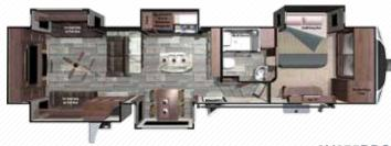
3X375RDS Ext. Length: 42'8" Hitch Weight (lbs): 2,710 Unloaded Wt. (lbs.): 13,110 GVWR: 16,470 Fresh Water (gal): 85 Gray Water (gal): 82 Black Water (gal): 41
