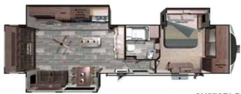
3X378RLS Ext. Length: 40'3" Hitch Weight (lbs): 2,310 Unloaded Wt. (lbs.): 12,180 GVWR: 15,990 Fresh Water (gal): 85 Gray Water (gal): 57 Black Water (gal): 41
