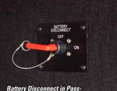
Battery Disconnect in Pass-Thru Storage Area
