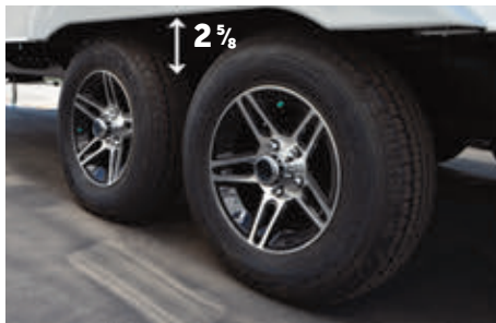
Available Chassis Lift Kit Provides an Additional 2 5/8" of Clearance
