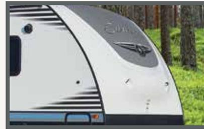
**TRAVEL TRAILER GEL-COAT FIBERGLASS CAP**
