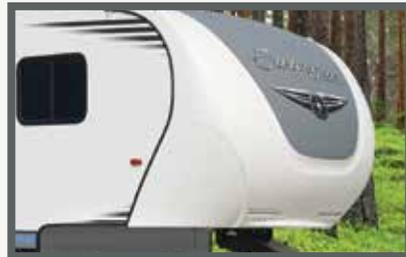
**FIFTH WHEEL GEL-COAT FIBERGLASS CAP**
