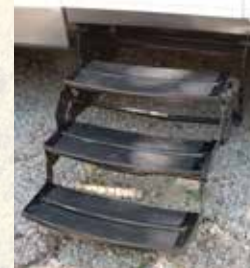
Radius entry steps give you larger step treads and fewer sharp corners
