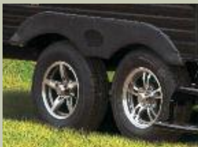
Tandem axles enhance stability
