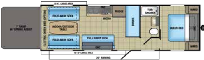
OCTANE SUPER LITE | 272 OPTIONS: A, B Ext. Lgth: 33' 11" Ext. Ht: 144" Unloaded Wt (lbs.): 7,050 Sleeps: 8-9
