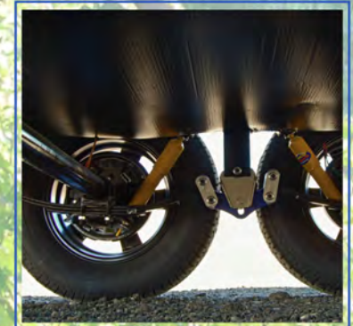
Heavy Duty Axles with Off-Road Brake System & 15" Mud Flaps
