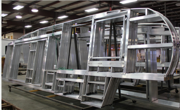
Voyage Lite features aluminum framing laminated with block foam insulation, true gel coat fiberglass exterior, and designer interior décor panels.
